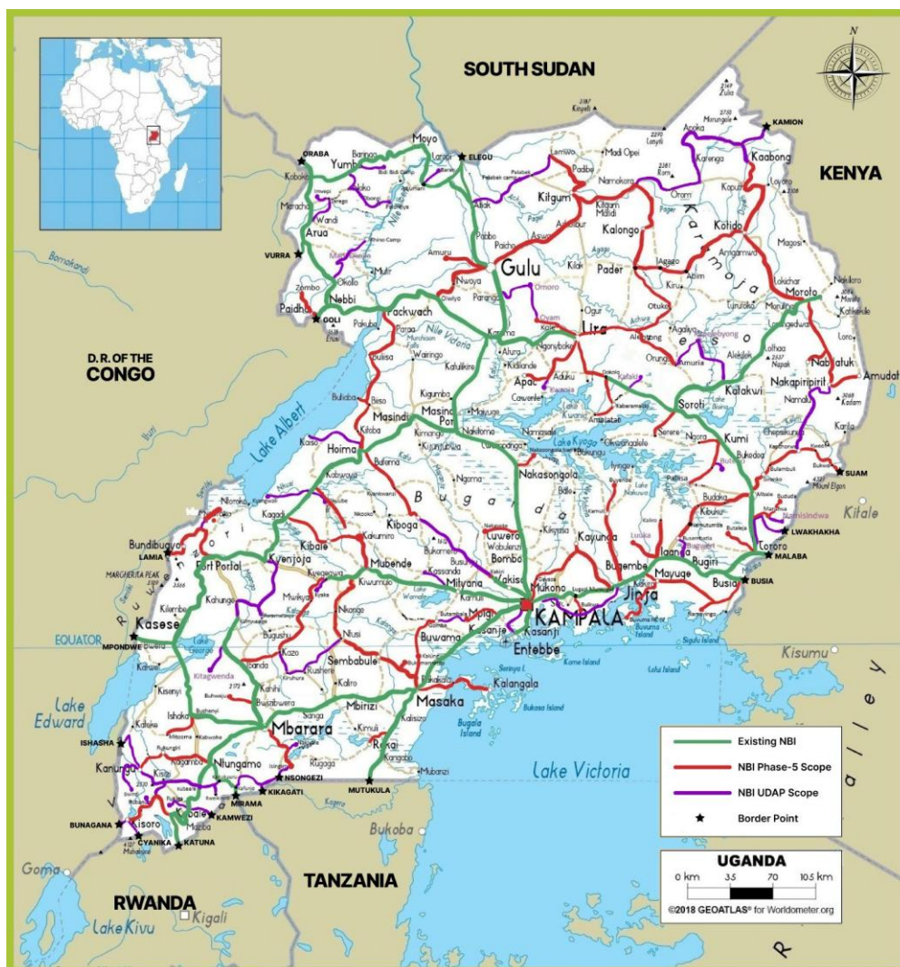
Figure 12: NBI coverage map showing completed and planned fibre developments
