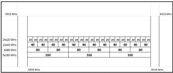
Figure 1. Channel Plan for the 6GHz band
